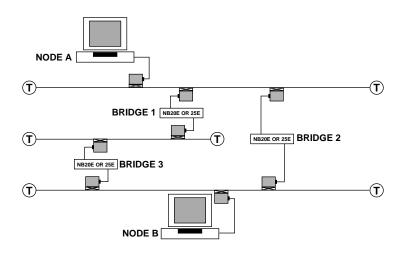
Figure 1-2 Multiple Bridging Environments
